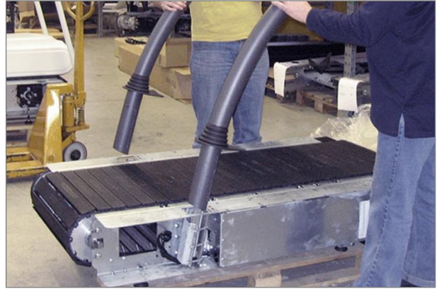
Fig. 27 Desmo assembly, inserting tubes
