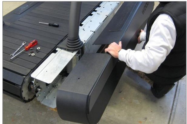
Fig. 35 Desmo assembly, side covers
