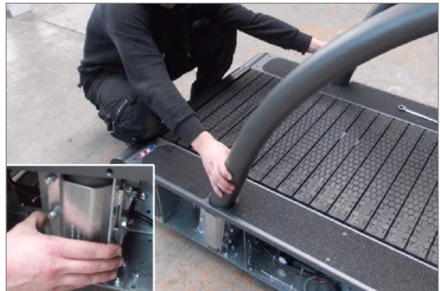
Fig. 18 4Front assembly, inserting tubes
