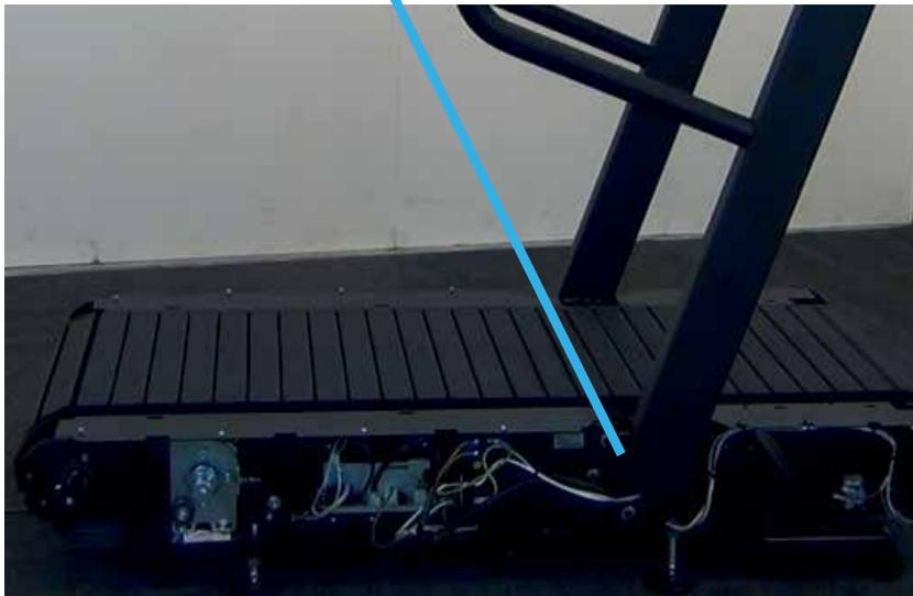
10. Remove the 3 screws (40), both on the right and on the left side of the equipment. (TOOL: 8 mm Allen wrench)
