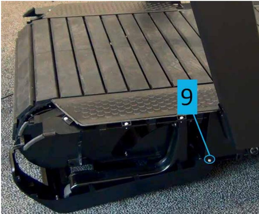
4. Remove the screw (9). (TOOL: medium Phillips screwdriver)
