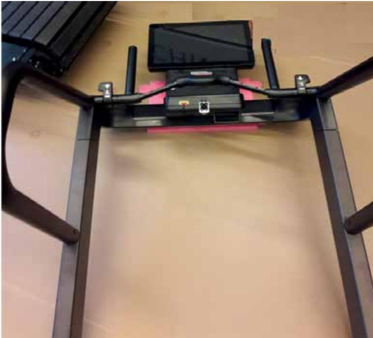
12. Remove the upright unit with the incorporated display from the equipment, and place it on the ground.
