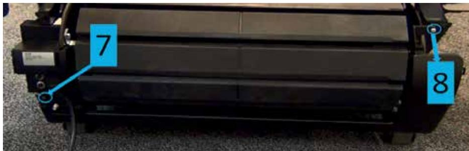
3. Remove the 2 front screws (7) and (8). (TOOL: medium Phillips screwdriver)
