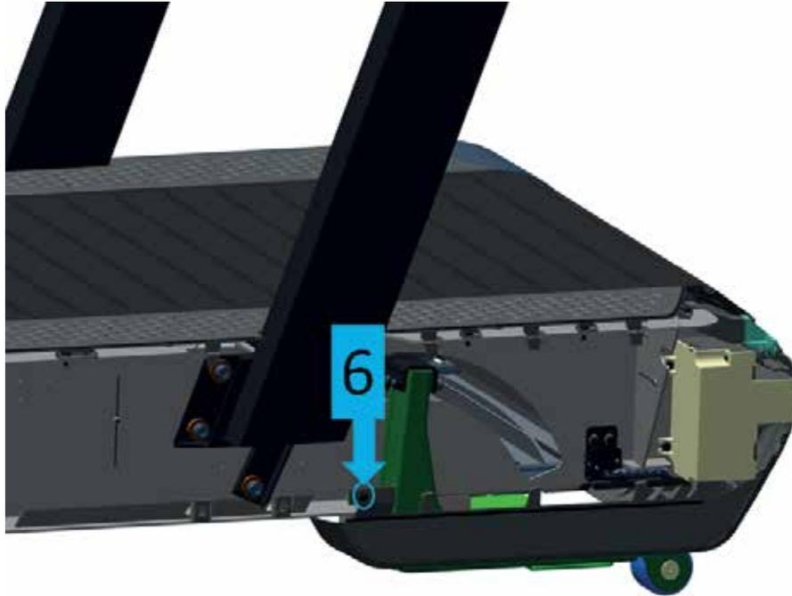
2. Remove the screw (6). (TOOL: medium Phillips screwdriver)
