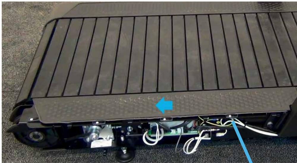
3. Push the footrest guard towards the rear part of the equipment, to release the screws from the eyelets.
