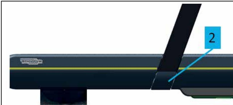
1. Remove the interlocked guard (2), pulling it towards the outside of the equipment.
