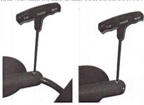
2. Notice that the bars cross over one another. This requires that you remove the bar that is the lower of the two. Do this by first loosening the set screws from the bottom of the bar (5/32'') Allen, this will allow you to slide the arm off of the lower rod end.
