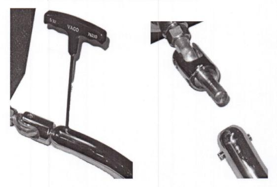
3. After sliding the arm off of the lower rod end, loosen the bolt that is holding the bar at the top of the machine. Do this, by slackening the  $\frac{3}{4}$ " back-up nut then loosen the rest of the way with the  $\frac{5}{8}$ " wrench. The rod ends have been adjusted at the factory to a certain length, this length must be noted when removing the rod end from the upper part of the bar.
