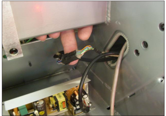
2 of the 3 console cable connections at the motor tray (the other is the coax cable).
