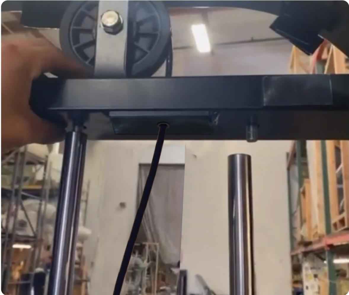
**STEP 6. INSTALL THE WEIGHT SELECTOR PIN AND REATTACH CABLE TO THE TOP PLATE AND THEN STORE WEIGHT ADAPTERS ON THE CHROME BRACKET AT THE TOP SO THAT THE CABLE CAN BE TIGHTENED AND ADJUSTED**
