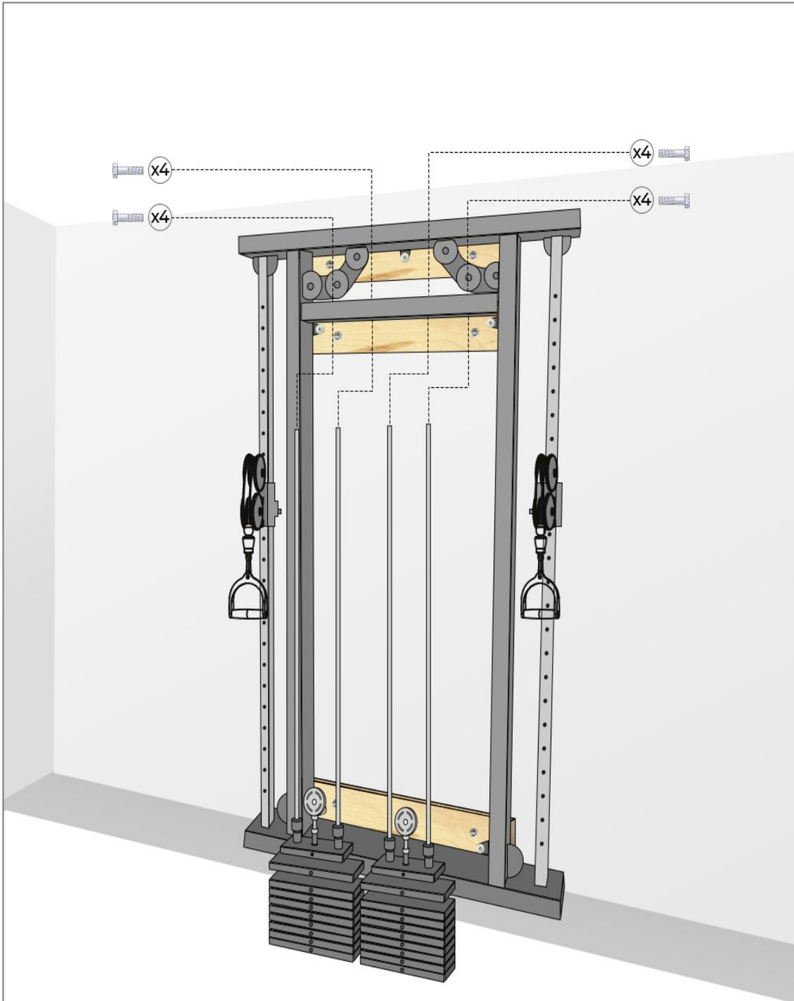
6) Install the weights. The large weights will go in first on each side evenly while the small weight goes in last.
