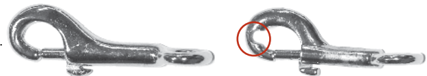
Figure 2: Good snap: no wear on hook. Bad snap: excessive wear on hook.
