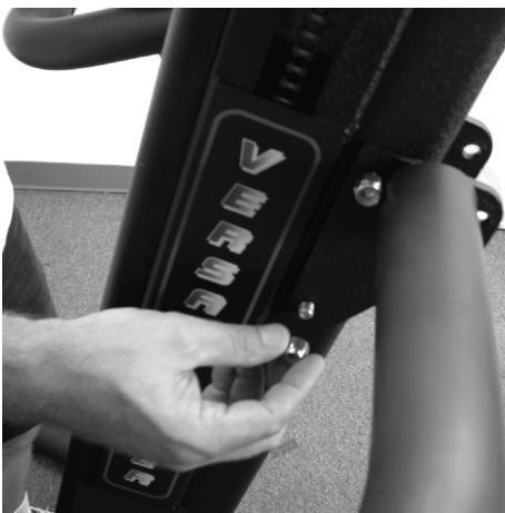
Loosely attach two 3/8" lock nuts nearest to the inside center of machine.
