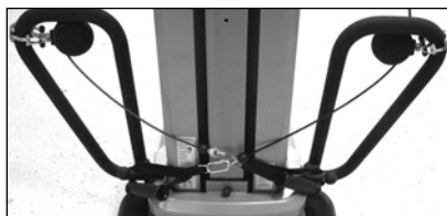
Figure 2: GTS® - Loop the handle straps around the opposite LAT bar pull pin as shown below.
