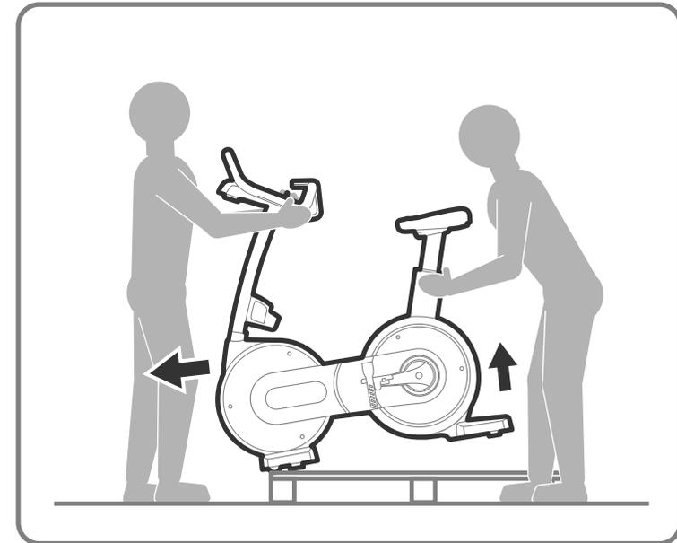
The equipment has two fixed front wheels. To move the equipment, lift it up slightly, as shown in the illustration, and push it forwards and backwards.
