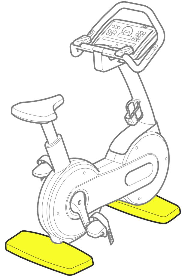
**Bases:** support the equipment frame and components.
