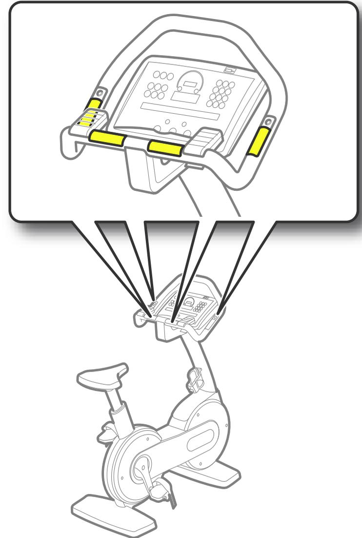
**Handlebar:** this can be held by the user during the workout. The 700 and 700 SP versions have **sensors** for monitoring the heart rate (hand sensor) and the **Fast Track Control** to change the effort level.
