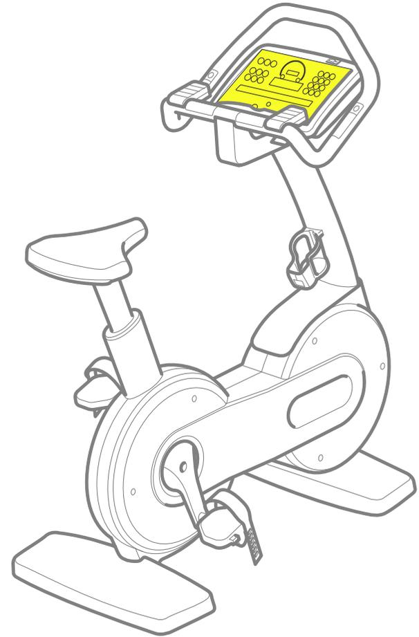
**Control panel:** controls all available functions, from setting up workout programs to viewing messages and related workout information.
