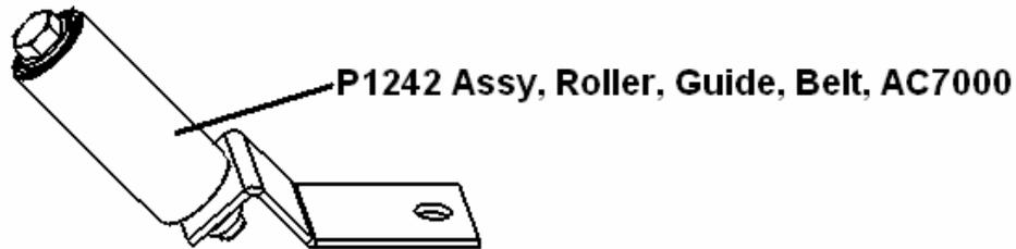
6. With a 9/16" wrench, remove the left side, front roller bolt. Loosen the right side, front roller bolt far enough to disengage the bolt threads from the roller threads. Rotate the right side of the front roller under the deck and belt. This will loosen the motor belt on the left side of the front roller and make it easy to slide off. Rotate the front roller approximately 90° from its original position. Pull the roller out from under the treadmill.
