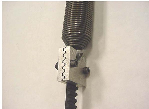
4. Remove the return spring from the other belt clamp. Remove the bolts that fasten the belt clamp to the belt and remove the belt from the clamp.
