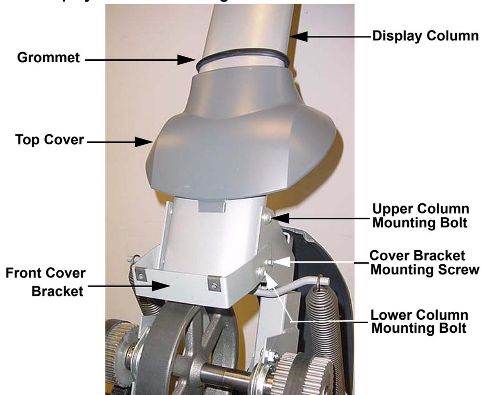
12. Fasten the display housing to the display column with the four screws removed in step 6.
