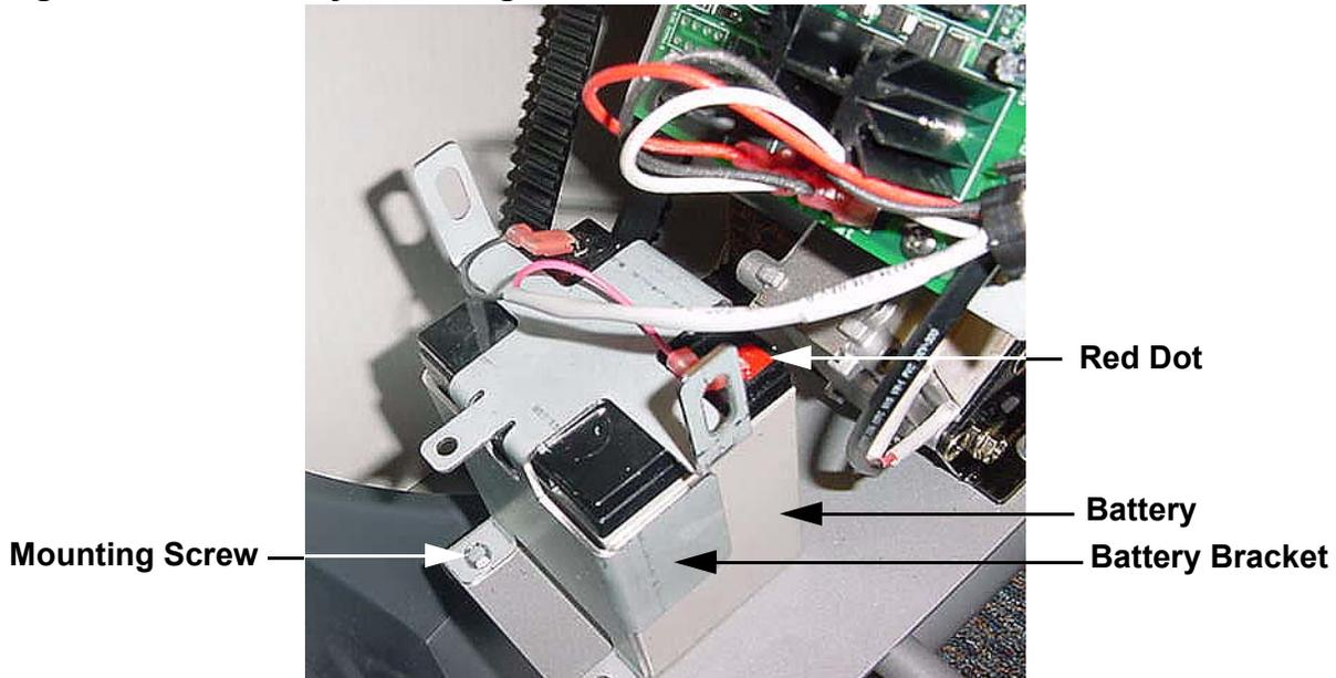
3. Remove both of the battery bracket mounting screws. Carefully, remove the battery bracket from the battery. Care must be taken to avoid touching the battery terminals with the battery bracket.
