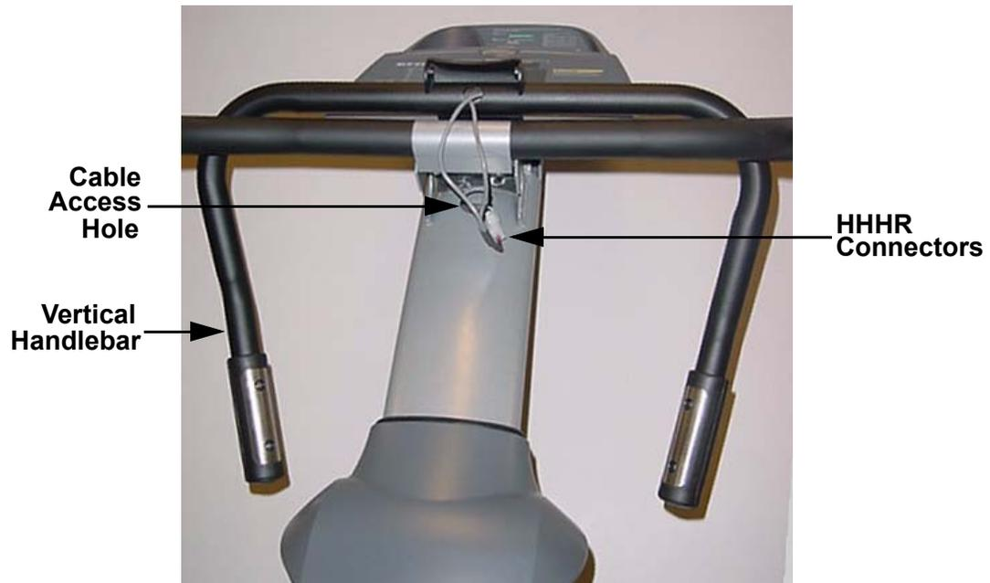
3. Disconnect the hand held heart rate (HHHR) connectors. Remove the vertical handlebar assembly.
