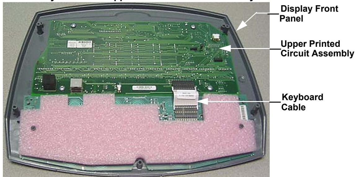
5. Use the C776i, if the **ERROR 05** or **STUCK KEY** message is still being displayed, replace the upper printed circuit assembly per Procedure XX.
