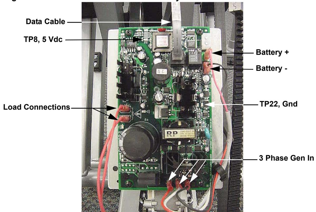
8. The following A.C. voltage readings will be measured on the **3 PHASE GEN IN** terminals. While the C776i is in use, perform the same A.C. voltage reading between the red and black, red and white and black and white wires. All three voltage readings should be approximately 90 Vac at 60 steps per minute. See Diagram 6.4.
