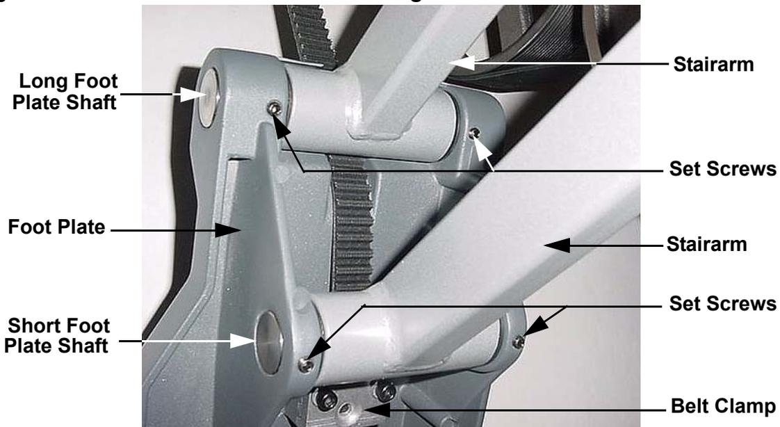
3. While supporting the foot plate, remove both foot plate shafts and remove the foot plate.
