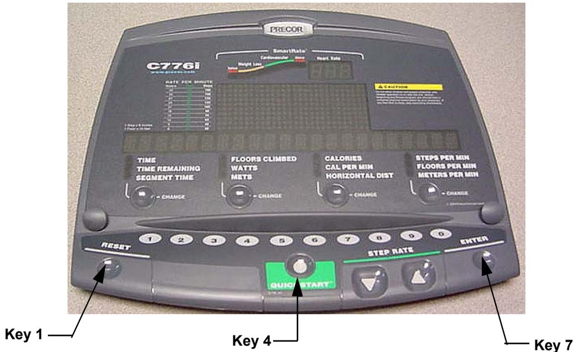
2. The message **INFORMATION DISPLAY** will be displayed for two seconds and then **ODOMETER** for two seconds. The total number of floors climbed will be displayed as **XXX FLOORS**. Press the **ENTER** key to continue to the total time display.
