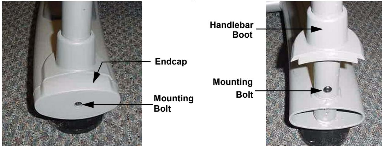
3. Remove the handlebar mounting bolt.
