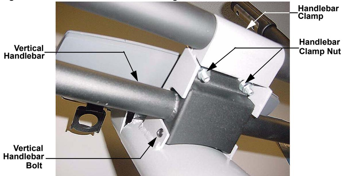
2. While supporting the vertical handlebar, remove both handlebar clamp nuts. Carefully, lower the vertical handlebar and then rotate it and set it on the left and right handlebars as shown in Diagram 7.9.
