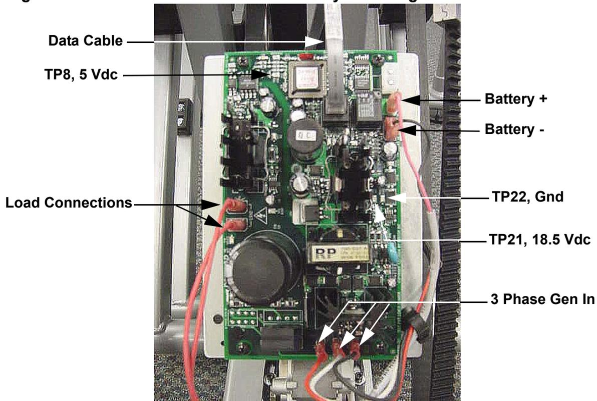
4. Set the replacement lower printed circuit assembly in its mounting position and fasten it with the four screws removed in step 3.
