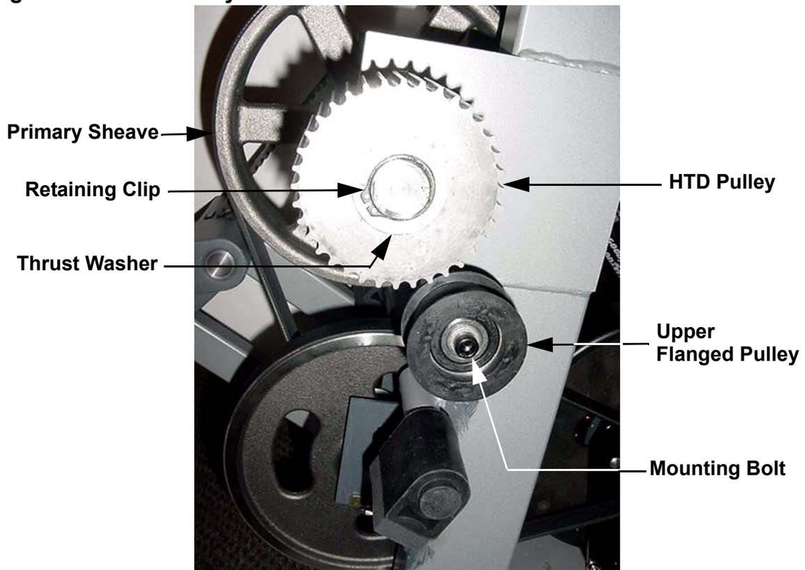
5. Remove the retaining clip from the HTD pulley. Remove the thrust washer from the shaft. Slide the HTD pulley off of the shaft. Verify that there are three thrust washers, one wave washer and another thrust washer remaining on the shaft.
