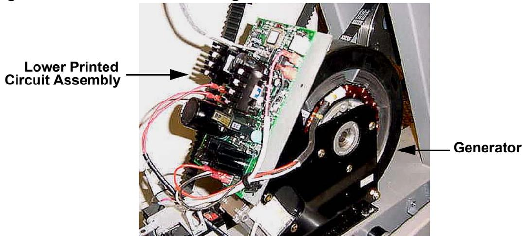
4. Remove the four screws that retain the lower printed circuit assembly. Remove the lower printed circuit assembly and set it on a static safe surface.
