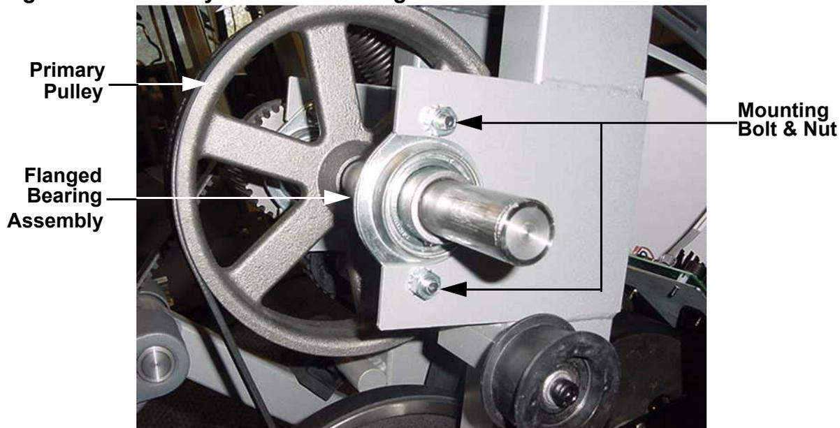
9. Slide the primary sheave out the frame and remove it from the primary belt.
