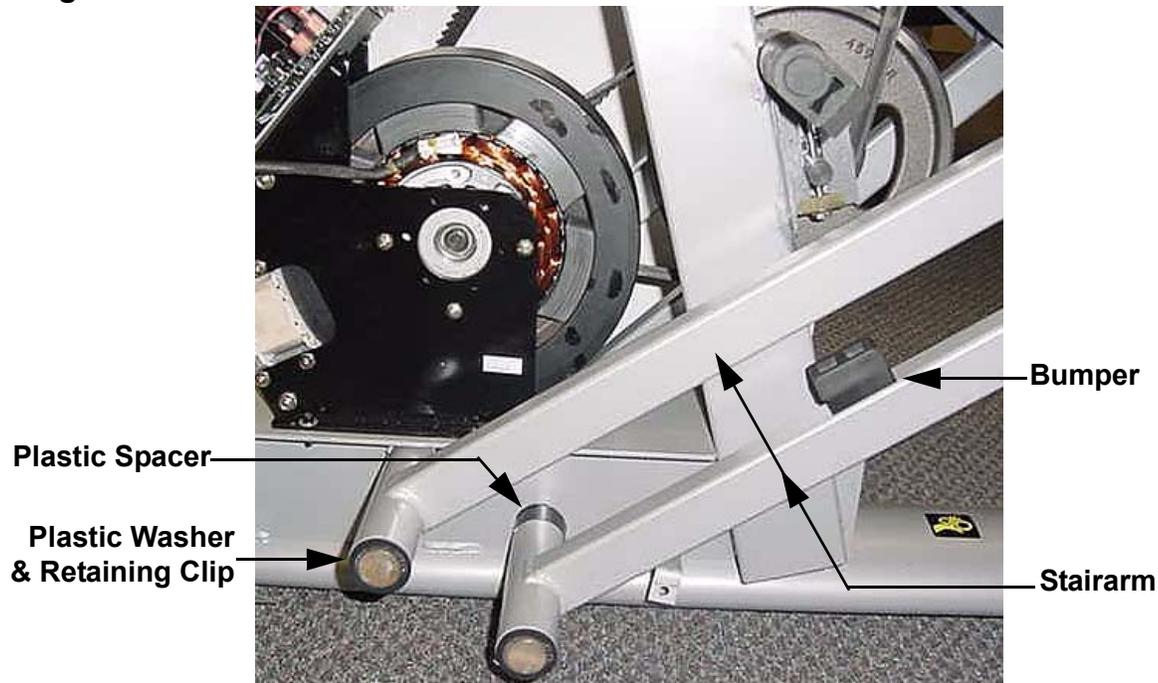
3. Remove the stairarm. If the lower stairarm is being replaced, remove the bumper from the stairarm and mount it on the replacement stairarm.
