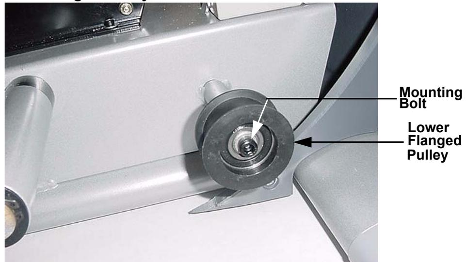
5. Set the replacement flanged pulley at its mounting position and fasten it with the bolt removed in step 4. Torque the mounting bolt to 120 inch pounds.
