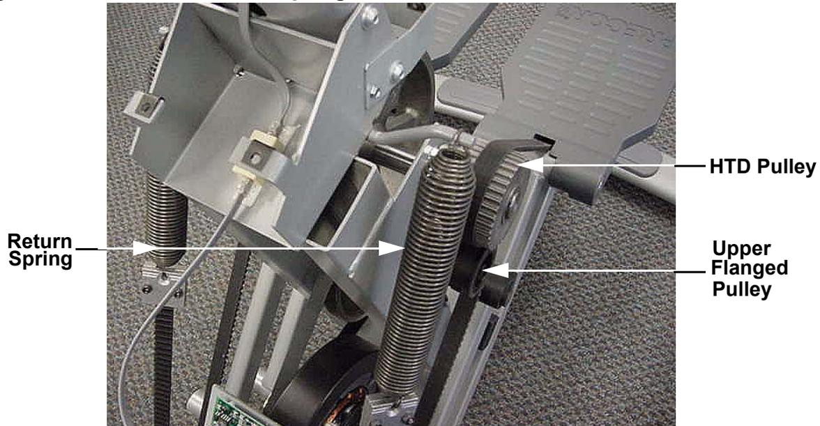
3. Support the stairarm and remove the stairarm belt from both flanged pulleys and the HTD pulley.
