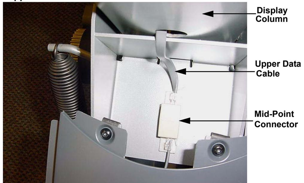
6. Remove the four screws that fasten the display housing to the display column. See Diagram 7.18. Carefully, remove the display housing from the display column while extracting the data cable and heart rate cable from the display column.
