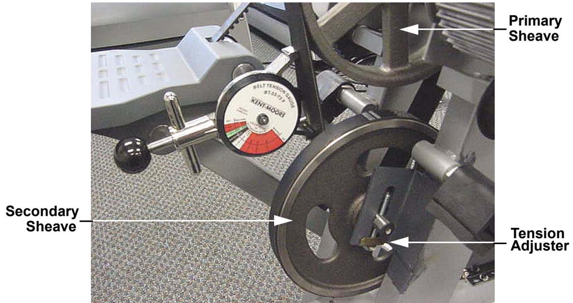
3. If necessary, adjust the primary drive belt tension using the two tension adjusters (one on each side of the secondary sheave) until the tension gauge reads approximately 100 pounds. There are locking tabs on the tension adjusters that must be straightened in order to turn the adjuster bolts. See Diagram 7.7. Bend the tabs back into the locking position when the belt tension adjustments are complete.
