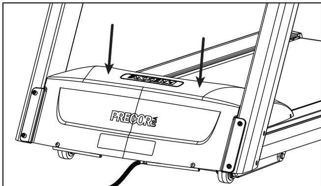
**9** Before using the unit, make sure it is level. If adjustments are needed, adjust one rear foot at a time. Do not raise the unit more than  $\frac{3}{4}$  inch (2 cm) from the floor.
