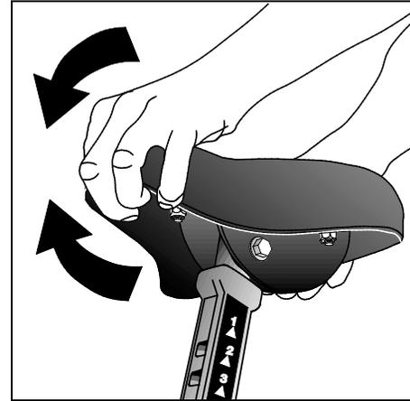
**Figure 7: Tilting the seat forward or backward**
