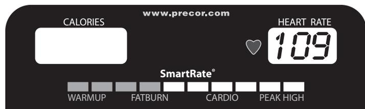
Heart rate and SmartRate® features are available when you wear the chest strap or grasp both touch-sensitive grips. When a heartbeat is detected, the HEART RATE display shows your heart rate and, if your age has been entered, the SmartRate LED blinks and indicates your target zone.
