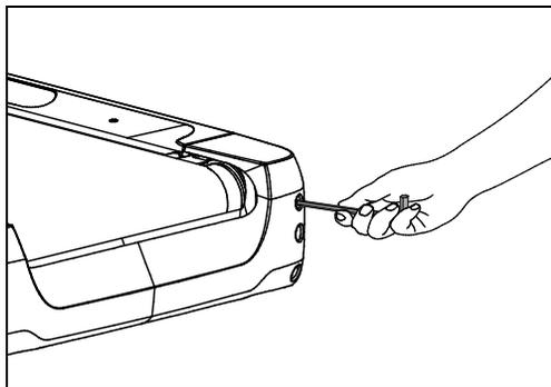
**Figure 5: Location of the adjustment bolt**
