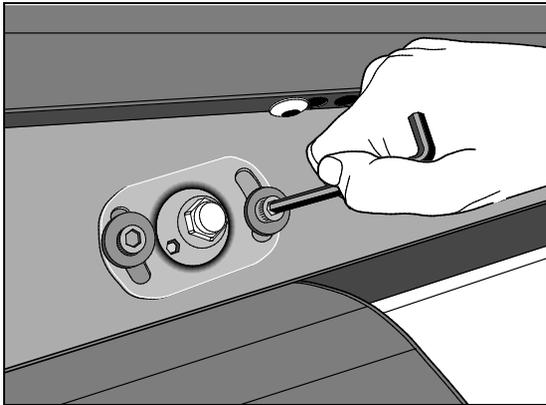
**Figure 8: Loosening the two adjustment screws**
