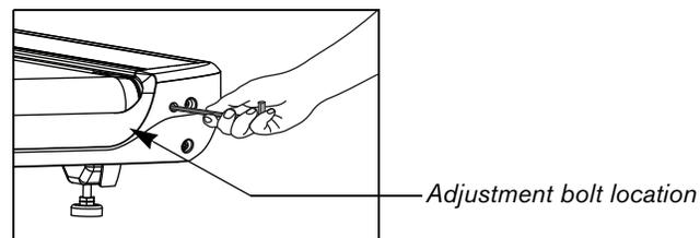
To determine left and right, stand at the rear of the treadmill and face the display. Make all belt adjustments on the **right rear corner bolt** using the 1/4-inch hex key.
