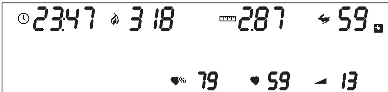
The top portion of the standard console is an LCD which prompts you to enter important information, dynamically displays all of the important workout data, and highlights aspects of your workout such as upcoming intervals and resistance changes. Watch the display as you set up and progress through your workout—it will guide you, motivate you, and reward you with summary information at the end of your session.
