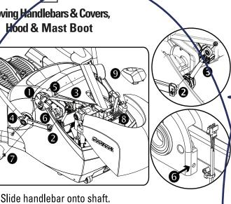
② Optional—adjust handlebar reach +/- 2.4" (61mm): Remove bolt, reposition shaft and spacer (top hole is longest reach), and re-install.
