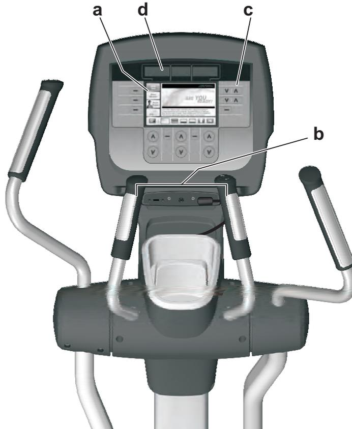
**a. Touchscreen Display:** The Touchscreen Display (the LCD screen) allows the user to choose, set up, and monitor a workout.
