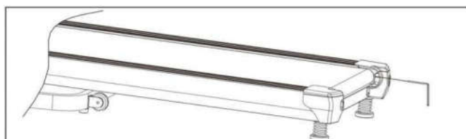
Adjust running belt to back of treadmill on both sides.
