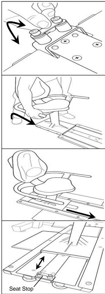
**Seat Stop:** Must be lowered to allow seat onto Baseplate track.
