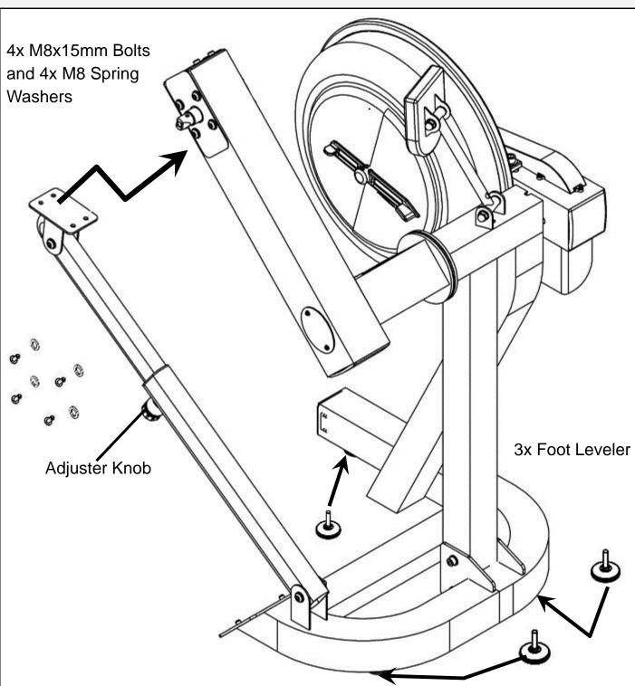
Remove contents from box. Attach telescoping tube to the underside of the control arm using **4x M8x15mm bolts[5]** and **4x M8 spring washers[16]**.
