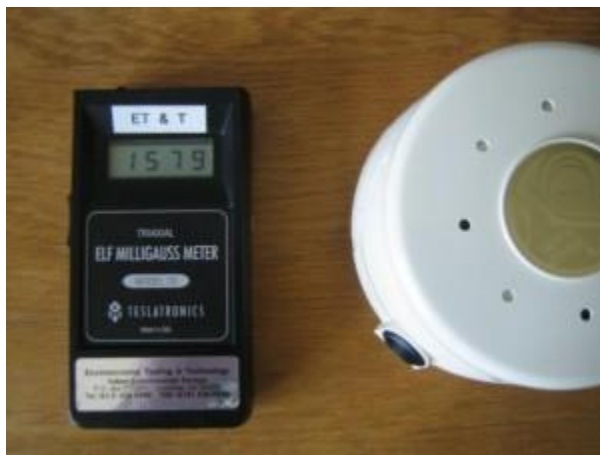
High field next to an air filtration device
