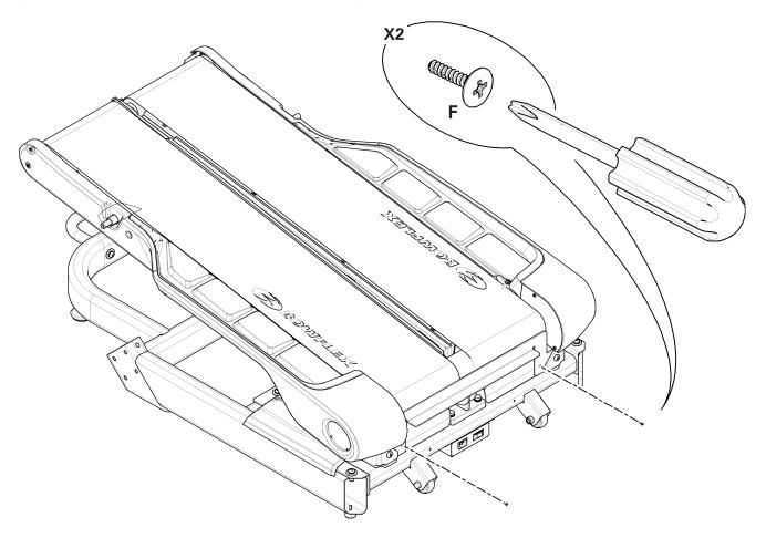
Step 5: Attach Junction Covers and Uprights to the Console/Handlebar Assembly
