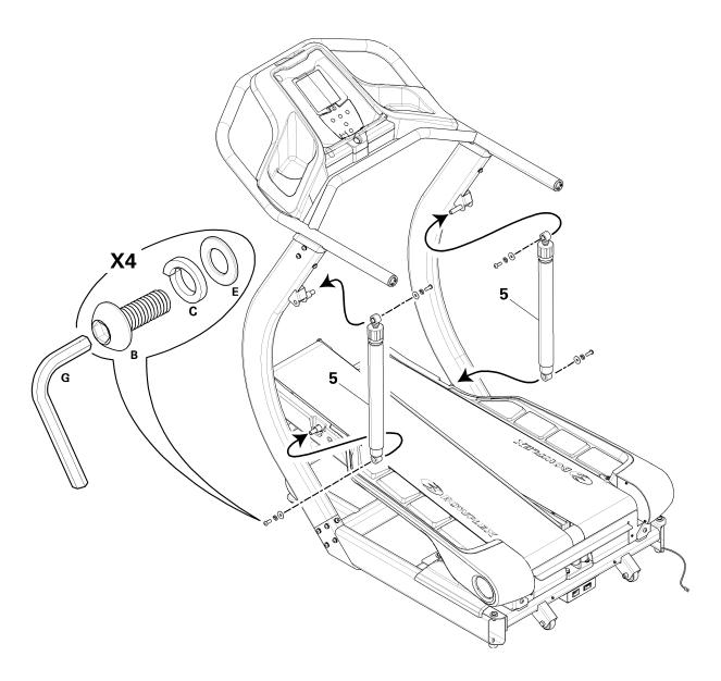
**Step 9: Connect the Console Cable to Rear of Machine**
