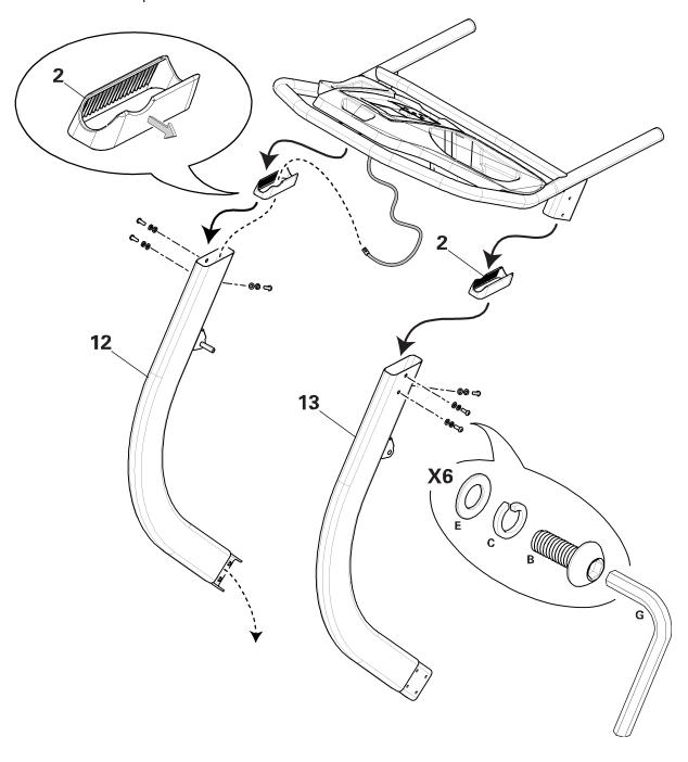
Step 6: Run the Console Cable through the Base Assembly
