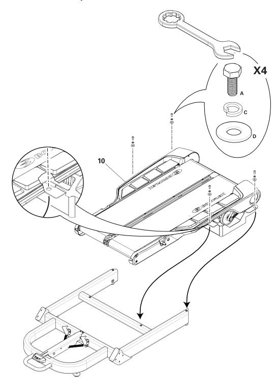
**Step 3: Attach Motor Cover to Base Assembly**
