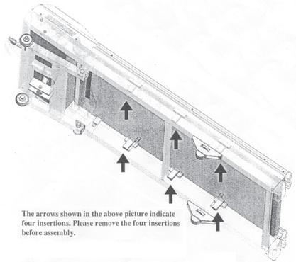
The arrows shown in the above picture indicate four insertions. Please remove the four insertions before assembly.
