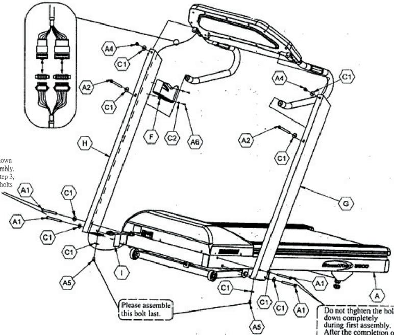
Do not tighten the bolts down completely during first assembly. After the completion of step 3, then you may tighten the bolts completely.
